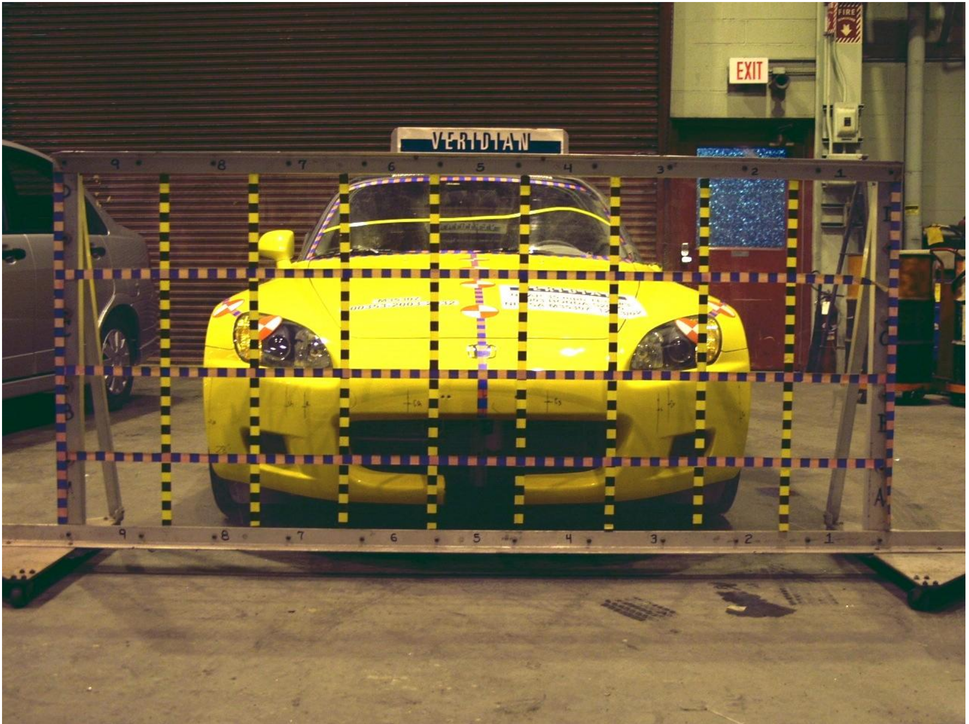
Figure A-1 LOAD CELL LOCATIONS
